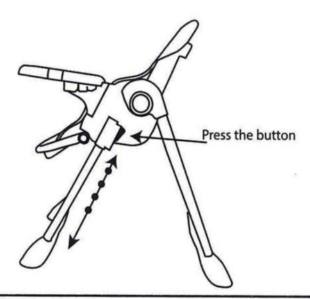
Step 11: Fold the chair: Simply press both buttons on the legs as shown below to fold and unfold the chair.
