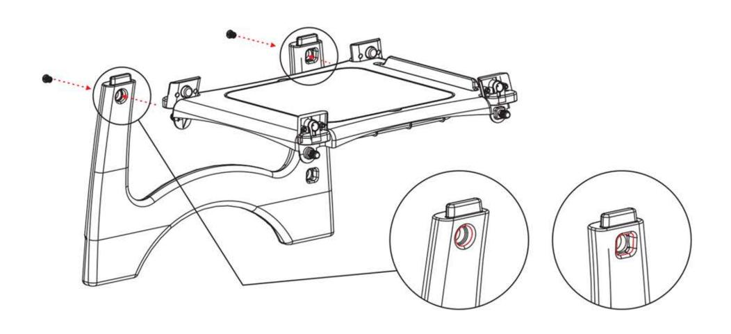
4. Buckle the long pedal plate into the left foot plate, and screw into 2 nuts.
