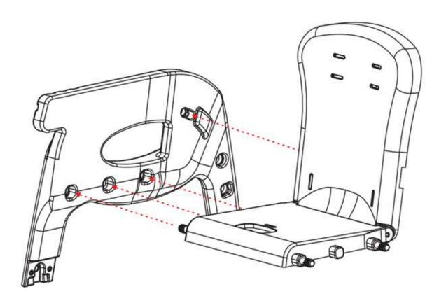
2. Buckle the pedal plate into the left of seat, and screw in 2 nuts.
