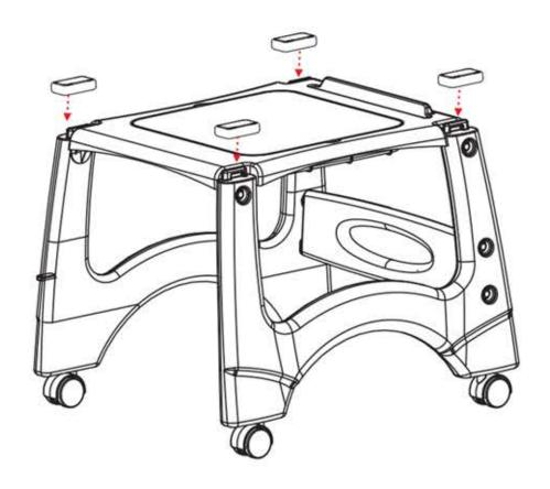
Disassemble plates as require. Hold the handle with both hands just pull the plate out.
